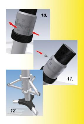
10. Set and adjust Nonius, considering ring gauge measurement ± linearity error according control certificate. Finally fix Nonius slotted screw slightly.
